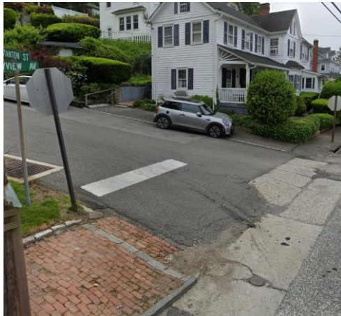
Bayview Avenue (Various materials & non-compliant curb ramps)
